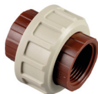
BOCCHETTONE in PP, ghiera filettata GAS, O-Ring in NBR
